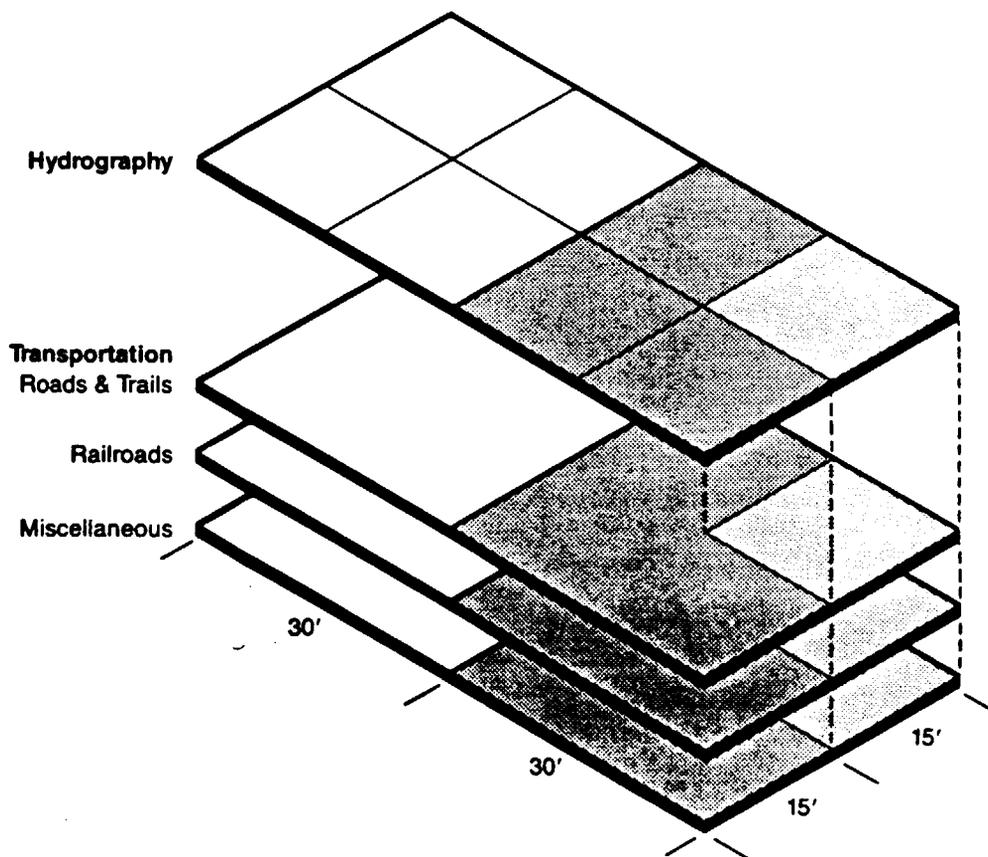
Diagram Showing Organization of Overlays and Files for the DLG Sampler
